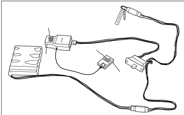
2. Turn on the receiver switch. Note that the LED's on both receivers should be flashing, indicating that the receiver is ready to bind.
