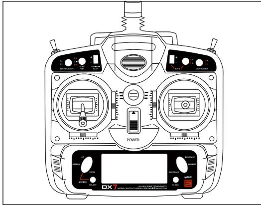
4. Press and hold the bind button on the back of the transmitter while turning on the power switch. The bind button should flash and within a few seconds the system should connect. The LED's on the receivers should go solid indicating the system has connected.
