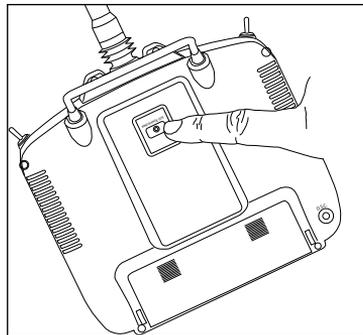
5. Remove the bind button and store it in a convenient place.
