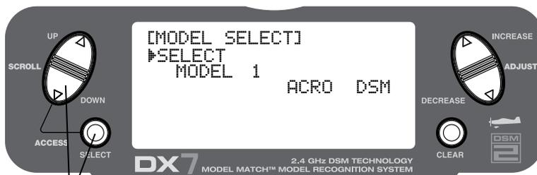
Hold while turning on transmitter to enter System Mode
