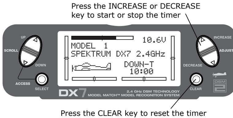
Press the **DOWN** and **SELECT** keys simultaneously to access the system mode.
