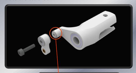
Make sure to leave approximately Ø4mm of material for the flat-mounting surface for proper installation of the Performance Tail Upgrade V2 series and support of the flanged radial-ball bearing.
