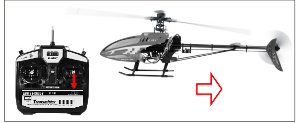
当升降操作杆向下推动时，直升机向后飞。 When the elevator stick is pushed downward, the helicopter flies backward.
