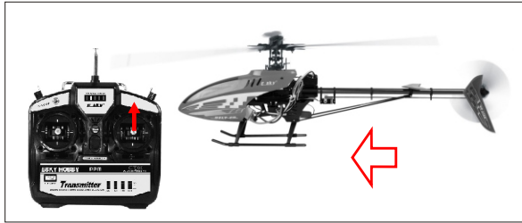
当升降操作杆向上推动时，直升机向前飞。 When the elevator stick is pushed forward, the helicopter flies forward.
