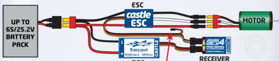
**DISCONNECT THE RED WIRE FROM THE ESC TO THE THROTTLE CHANNEL ON YOUR RECEIVER WHEN USING THE CC BEC (DISREGARD IF USING WITH PHOENIX HV CONTROLLERS)**
