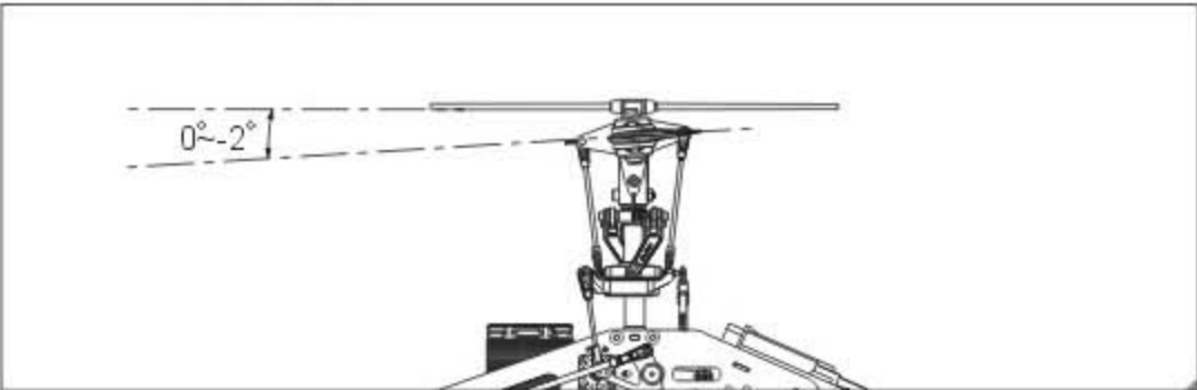
Stick position at low/Throttle 0%/Pitch0~-2° 搖桿低速/油門0%/Pitch0~-2°
