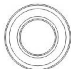
Bearing 軸承 (φ 10x φ 19x5mm) x 2
