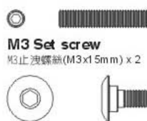
M3 Set screw M3止洩螺絲 (M3x15mm) x 2
