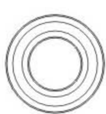
Bearing 軸承 (φ 9x φ 17x5mm) x 1
