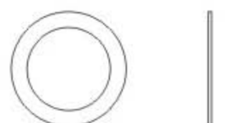
Spindle bearing spacer 橫軸軸承墊片(φ10xφ13.8x0.4mm) x 2
