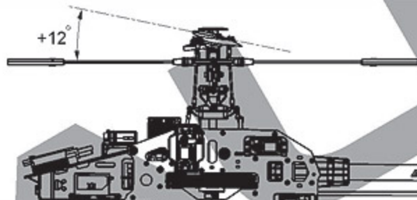
Stick position at high/Throttle 100%/Pitch +10°~+12° 搖桿高速/油門100%/Pitch +10°~+12°
