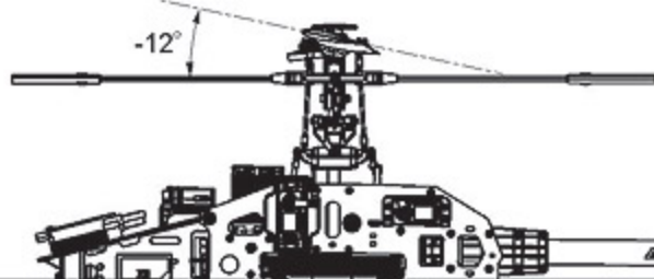
Stick position at low/Throttle 100%/Pitch -12° 搖桿低速/油門100%/Pitch -12°
