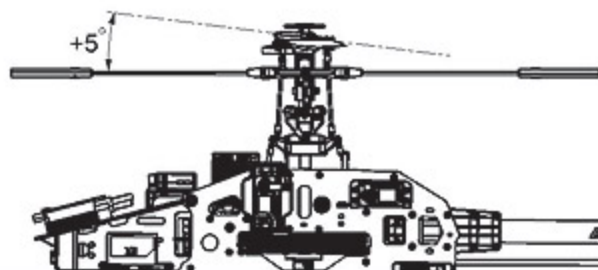
Stick position at Hovering/Throttle 60%~65%/Pitch +5° 搖桿停懸/油門60%-65%/Pitch+5°
