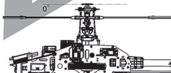
Stick position at middle/Throttle 85%/Pitch 0° 搖桿中速/油門85%/Pitch 0°
