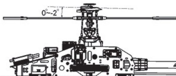
Stick position at low/Throttle 0%/Pitch 0°~2° 搖桿低速/油門0%/Pitch 0°~2°
