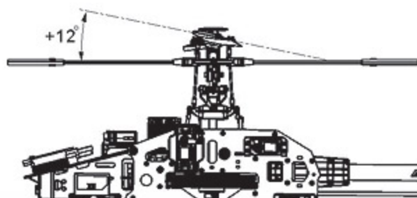
Stick position at high/Throttle 100%/Pitch +12° 搖桿高速/油門100%/Pitch+12°
