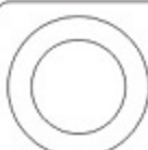
Bearing 軸承 (φ12xφ18x4mm) x 1
