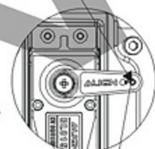
Use the outer hole 請鎖附於外孔
