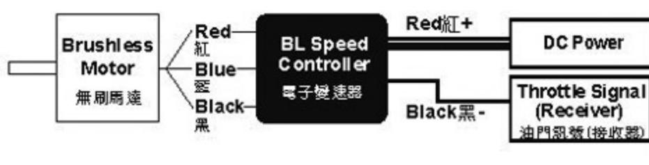
The motor rotates in different direction with different brand ESCs. If the wrong rotating direction happens, please switch any two cables to make the motor rotates in right direction.
