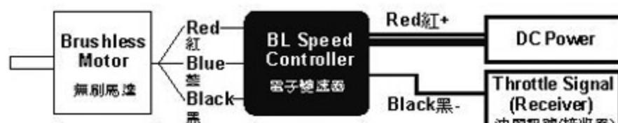
The motor rotates in different direction with different brand ESCs. If the wrong rotating direction happens, please switch any two cables to make the motor rotates in right direction.
