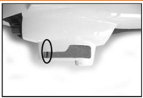
Insert the 4x55mm Carbon Rods into the specific position of the Gun Housing and secure it with glue. (This is used to prevent further retraction of the Retract System.)
