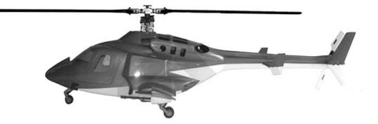
SpecificationsLength:728mmHeight:159mmWidth:268mmWeight:355gSuitable for ALIGN T-REX 450Nitro series
