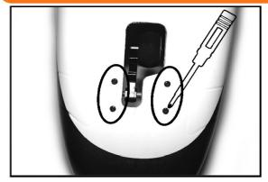
Use M3x10mm screws x4 with M3 Nuts to tighten the Front Retract System onto the fuselage body.
