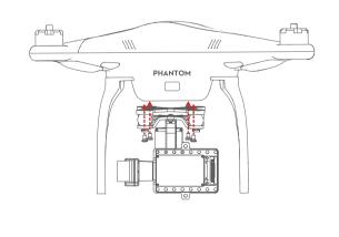
Mount the camera into the Camera Mounting Base of the gimbal and fix the camera by the Camera Fixed Mounting. Tighten the two M2.5x6.3 screws.
