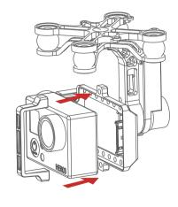
Assembly is finished. Make sure the Damper Unit is horizontally assembled and both damping boards are paralleled to the bottom of the aircraft, further to make sure the gimbal is precisely and firmly
