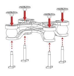
Tighten the two M2.5x5 screws to fix the gimbal to the Bottom Board of Damper Unit.
