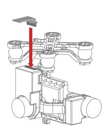
Tighten the four M3x5 screws to assemble the Top Board of Damper Unit to the bottom of aircraft. Make sure the Camera Mounting Base of the gimbal is pointing to the aircraft nose direction.
