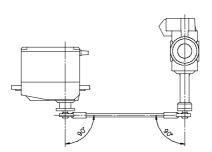
Locate the servo so that its output arm and the throttle pushrod are, as close as possible, directry in line with carburetor's throttle arm, as shown.
