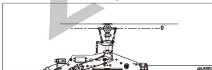
Stick position at middle/Throttle 60%~65%/Pitch 0° 搖桿中速 / 油門 60%~65%/Pitch 0
