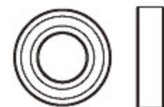
Bearing 軸承 (φ 12x φ 24x6mm) x 2
