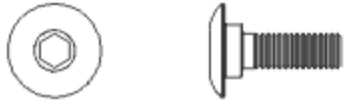
Socket button head collar screw 半圓頭內六角轉套螺絲(M3x8mm) x 8
