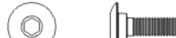
Socket button head collar screw 半圓頭內六角轉套螺絲(M3x8mm) x 6
