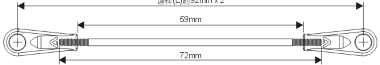
Linkage rod(E) Approx. 92mm x 2 連桿(E)約92mm x 2
