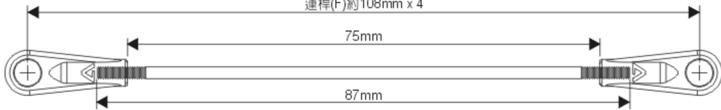
Linkage rod(F) Approx. 108mm x 4 連桿(F)約108mm x 4
