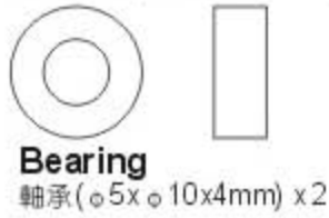
Thrust bearing 止推軸承(φ5xφ10x4mm) x 2
