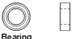
Bearing 軸承(φ4xφ7x2.5mm) x 2
