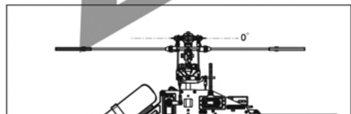
Stick position at middle/Throttle 85~90%/Pitch 0° 搖桿中速/油門85~90%/Pitch 0°
