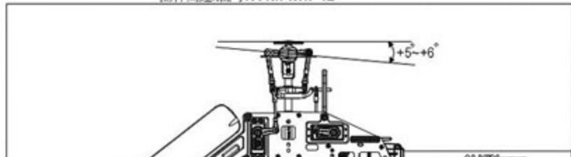
Stick position at Hovering/Throttle 65%~70%/Pitch +5~+6° 搖桿停懸/油門65%~70%/Pitch +5~+6°
