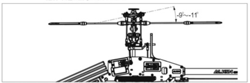
Stick position at low/Throttle 100%/Pitch -9° ~ -11° 搖桿低速/油門100%/Pitch -9° ~ -11°
