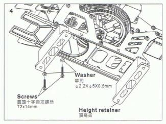
Remove the landing skid of Trex450 helicopter and fix the height retainer on T-REX bottom plate with screws T2x14 and M2 washers.
