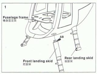
Apply AB glue at the marked position on the landing skid. Then insert to the fuselage and wait until dry.
