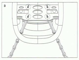
Use a diagonal cutting pliers to cut the protruding part and sandpaper to make it smooth.
