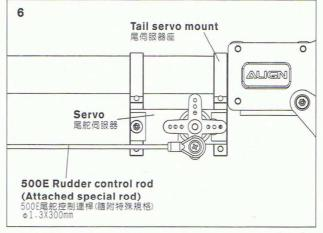
Install a tail servo on the tail boom as illustration and switch to 500E attached special rudder control rod  $_{\odot}$  1.3x300mm.
