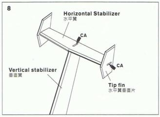
Apply some CA glue on the joints of horizontal stabilizer and tip fins and keep them vertical. Apply some CA glue on the joints of vertical stabilizer and horizontal stabilizer and keep horizontal.
