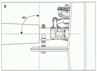
Adjust the fixing position of the height retainer and keep the center lines of the tail boom and the fuselage at the same level.
