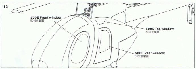
Assemble the front and rear windows on the fuselage as illustration (Recommend not assembling the rear windows to increase the airflow efficiency.)
