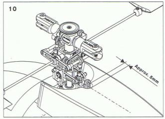
After Step 9, adjust the fixing position of the height retainer and make the main rotor head assembly at the center line of the fuselage. Note to keep 5mm gap between the anti-rotation bracket and the fuselage.
