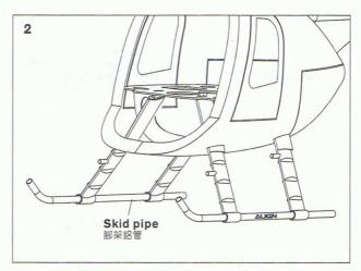
Insert the skid pipes (two pieces) into the front and rear landing skids as illustration.
