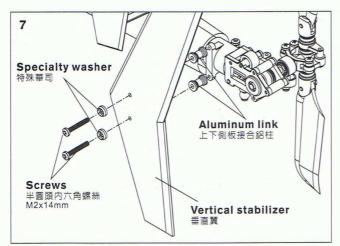
Assemble the helicopter into the fuselage and re-install the tail case and tail rotor assembly step by step. Then assemble the vertical stabilizer as illustration
