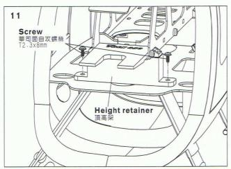
After the adjustment, fix the height retainer and the fuselage frame with screws T2.3x8mm.
